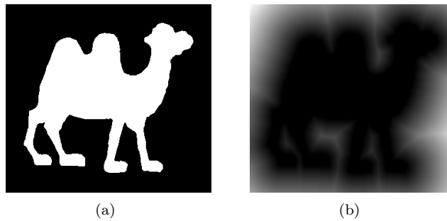
FIGURE 1 – (a) A binary image (on a cubical cellular space) and (b) its distance transform.
